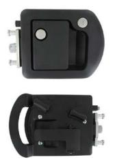
Tri*Mark's* NEW 060-1650 Motor Home Entrance Door Hardware with Dead Bolt is designed for RV motor home and fifth wheel trailer entrance doors and is a redesign of our 060-0650 Motor Home Entrance Door Hardware. It features easy installation with through sandwich mounting, a low profile plunger style latch which is compliant to FMVSS 206, a built-in dead bolt for additional security and is power lockable.
